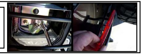
Step 11: Reinstall the four screws removed in step 1.
