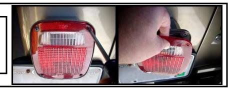
**Step 3:** Remove the 3 tail light assembly retaining bolts.
